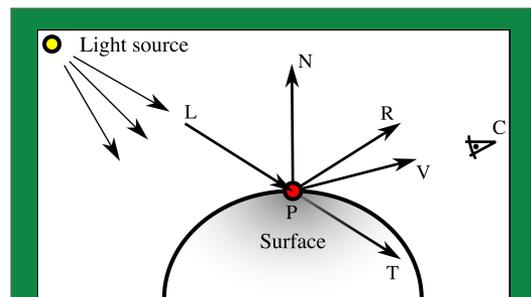
**Figure 4:** Incoming light (L) from a light source can get absorbed, reflected (R), or transmitted (T) when interacting with a surface point (P) before it reaches the camera/eye (C).
