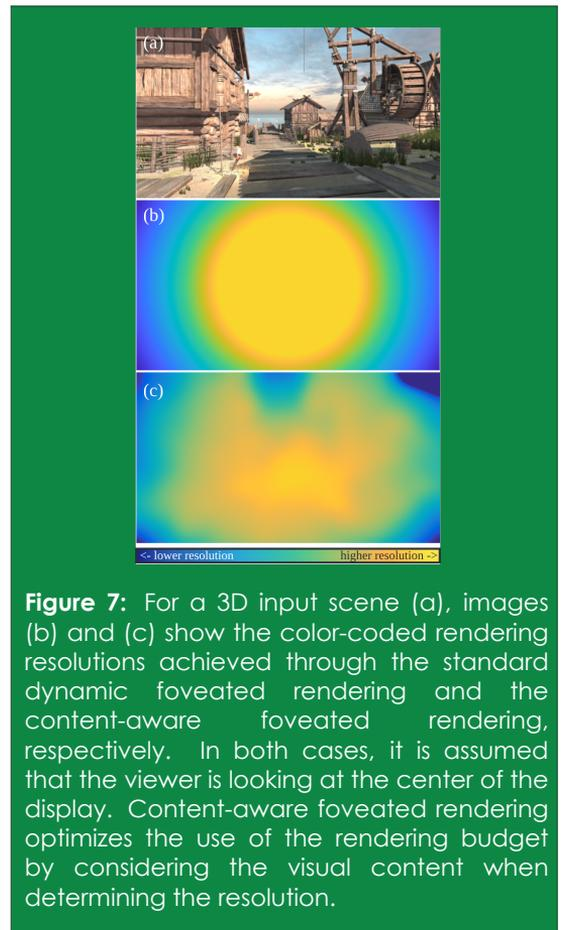
**Figure 7:** For a 3D input scene (a), images (b) and (c) show the color-coded rendering resolutions achieved through the standard dynamic foveated rendering and the content-aware foveated rendering, respectively. In both cases, it is assumed that the viewer is looking at the center of the display. Content-aware foveated rendering optimizes the use of the rendering budget by considering the visual content when determining the resolution.
