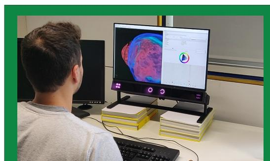
**Figure 6:** A foveated rendering system consisting of a desktop display and an eye tracker positioned beneath the display.
