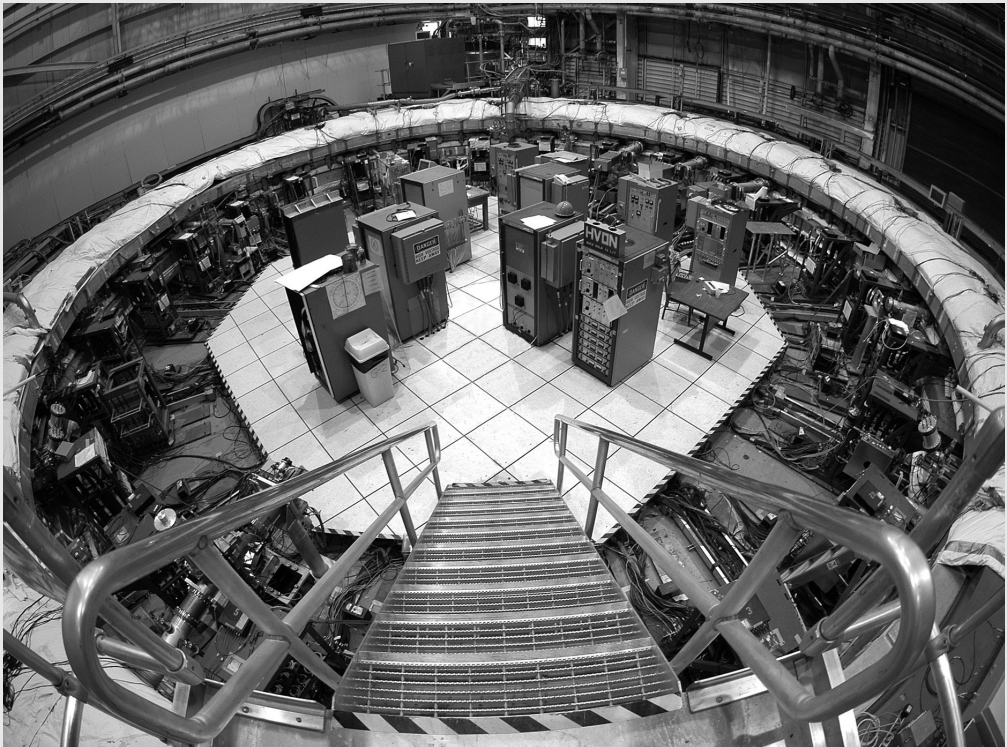
FIGURE 2 Brookhaven National Laboratory. The storage ring used for the measurements of the g-factor of the muon.
